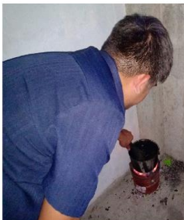
The plastic wastes were heated to a molten state, and combined with clean river sand, crushed glass bottles and shredded papers
