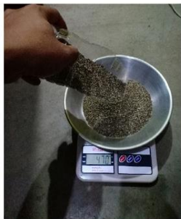
The amount of aggregate was measured through the use of digital weighing scale
